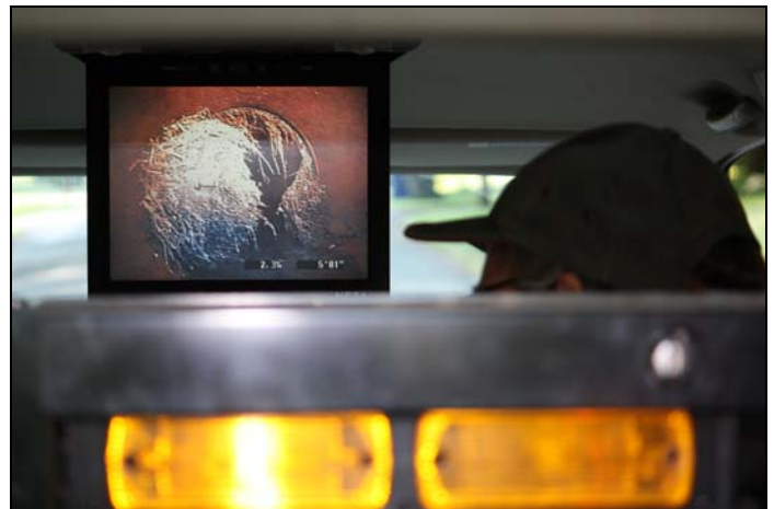
View from inside the control vehicle, showing root blockage.
