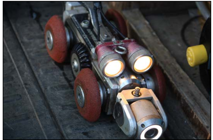
Sewer Line Camera ready to work.
